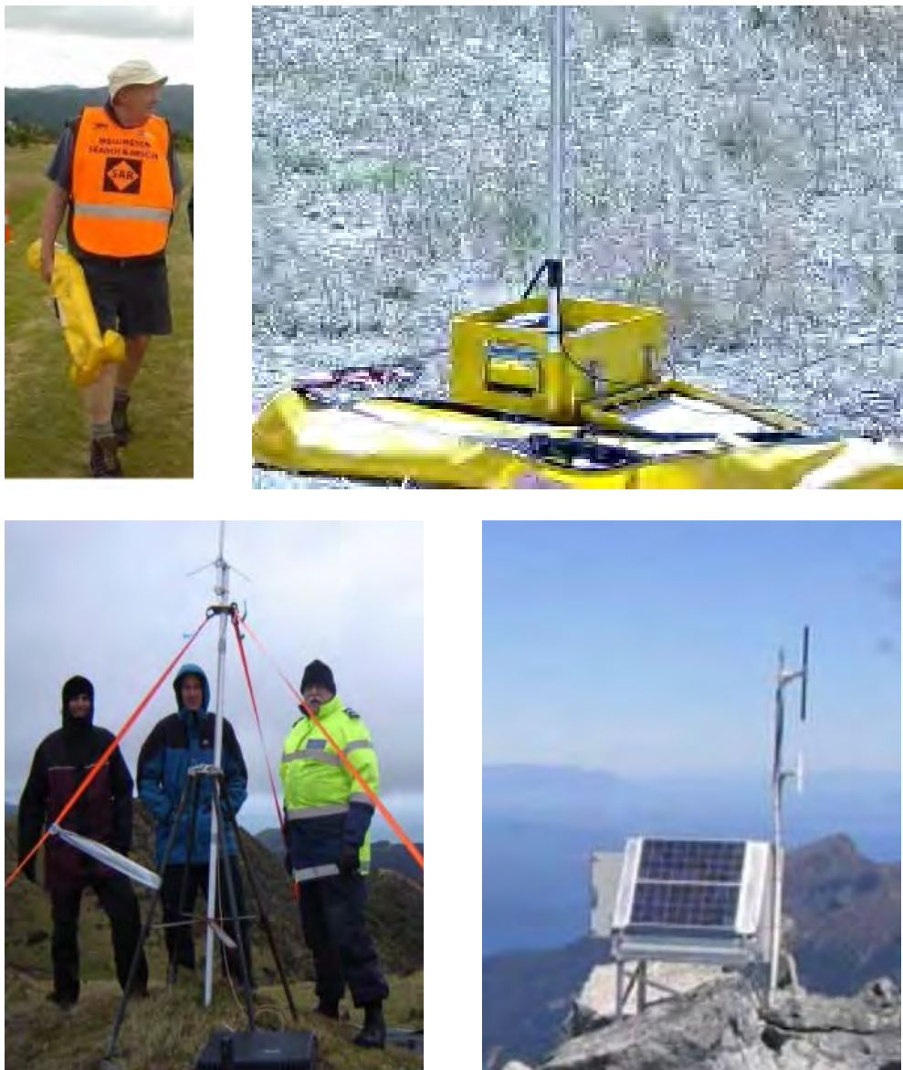
Figure 2: Police Portable Repeater equipment and aerial assembly
